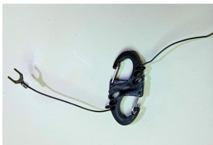
I use a **Carabiner** clip, get these on Amazon. Once you have the wire threaded (the 32'9" end at the start of the Carabiner) the rest is strain relief about an extra 2" that goes to the Antenna connection on the 49:1 transformer. See next photo.
