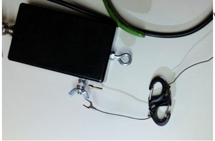
Clip Carabiner to eye bolt, and wire lug to antenna connection
