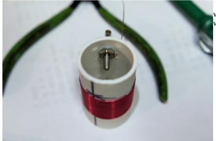
Here you see the Nut and Star washer installed, hold with small wrench or pliers and tighten screw
