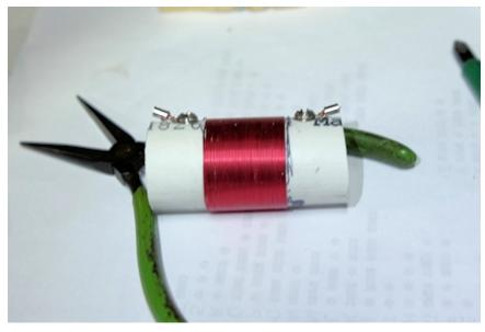
Let's make a loading coil for the 20m/40m short EfHW antenna element.
