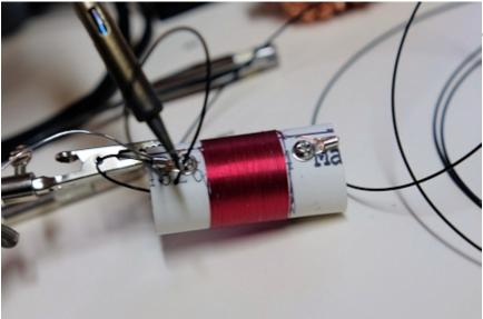
Now solder both antenna wire and coil wire to lug.
