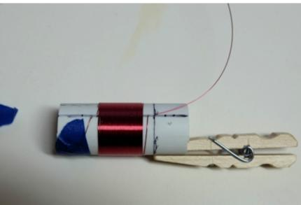
Once pulled taught the wire is locked in place and we can add other components to the complete the Loading Coil
