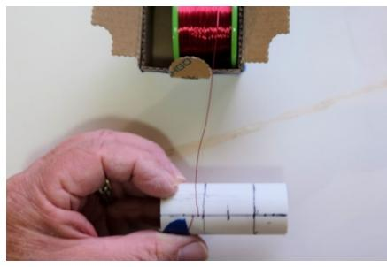
begin the wrap, notice under my thumb, I have used a piece of tape to keep the end of the wire from interfering with winding. The grip you see is used over the wire to keep tension and to keep the wire from unwinding, I rotate the core with my right hand. That line running from one end to the other is to keep track of the count.
