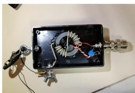
I used some bell wire to make this one, it shows some slight heating of the wire that is wound around the core, (I stress tested the unit) it will handle 100w, I only run 80w when out activating a park, just habit, but will on occasion run 95w.
