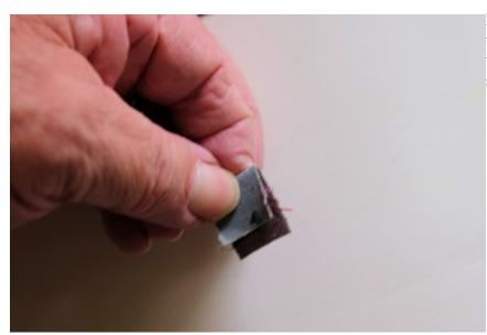
Now use the sand paper and draw the wire between the sand paper to remove the coating so it can be soldered.
