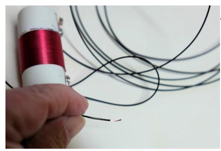
Remove ¼" of jacket to bare the wire, tin push into lug.
