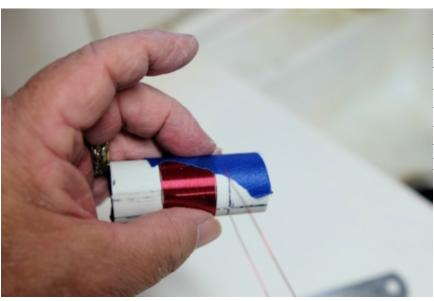
I have put tape on to hold the wire tension while I drill the two locking holes for this side of the core. We'll then tread the wire through the holes. Now is a good time to cut the end down to about 3" and sand the varnish coating off before threading it through the locking holes.
